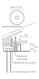
Note: The client is responsible for providing a robust 16mm (5/8") plywood backing or wood blocking to securely anchor to the structural substrate.
